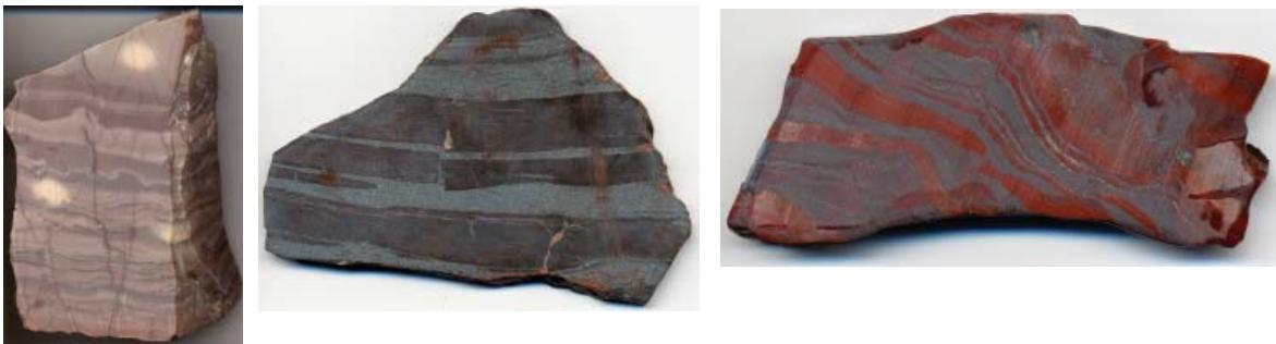
Figure 1: Samples of banded iron from the Lake Superior Banded Iron Formation. Iron (III) oxide ( \text{Fe}_2\text{O}_3 ) minerals can appear reddish-brown or gray depending on grain size cemented within the mineral. In either case, it is called hematite. Samples (a,b) are each about 3.5 inches long. Sample (c) is about 4.5 inches long. (a) Red hematite layers alternated with silicate layers stained with iron-bearing fluids. (b) Iron is contained in the shiny bands of specular (reflective) hematite. The iron is banded with shale (organic-rich ancient clays), metamorphosed to slate. (c) Here, the iron oxide appears as specular hematite, banded with quartzite — \text{SiO}_2 , deposited as sand and metamorphosed. The quartzite was stained red by iron-bearing fluids at deposition. (Samples and mineral descriptions provided by A. Joyal, Northern Michigan University)
