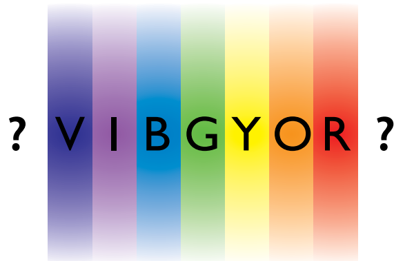
Figure 2: A sketch of colors in the visible spectrum. The order of colors from right to left can be remembered as “Roy G. Biv” (red, orange, yellow, green, blue, indigo, violet). There is an infinite number of colors smoothly varying from one end of the spectrum to the other. What colors go to the right and the left of the visible spectrum?
