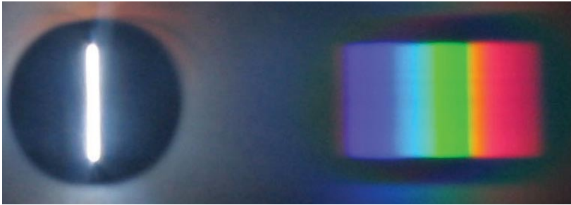
Figure 1b: Light from a clear, blue sky, viewed through a diffraction grating spectroscope. You can see the slit and the spectrum, off to the side.
